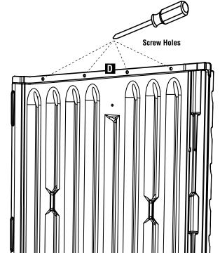
Connect Left Back (D) into dovetails of Repeat Left Side (C).
